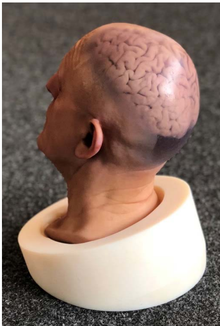
Translucent head model: multi-material 3D printing using the universal 3D printer drive Cuttlefish. | © Fraunhofer |
