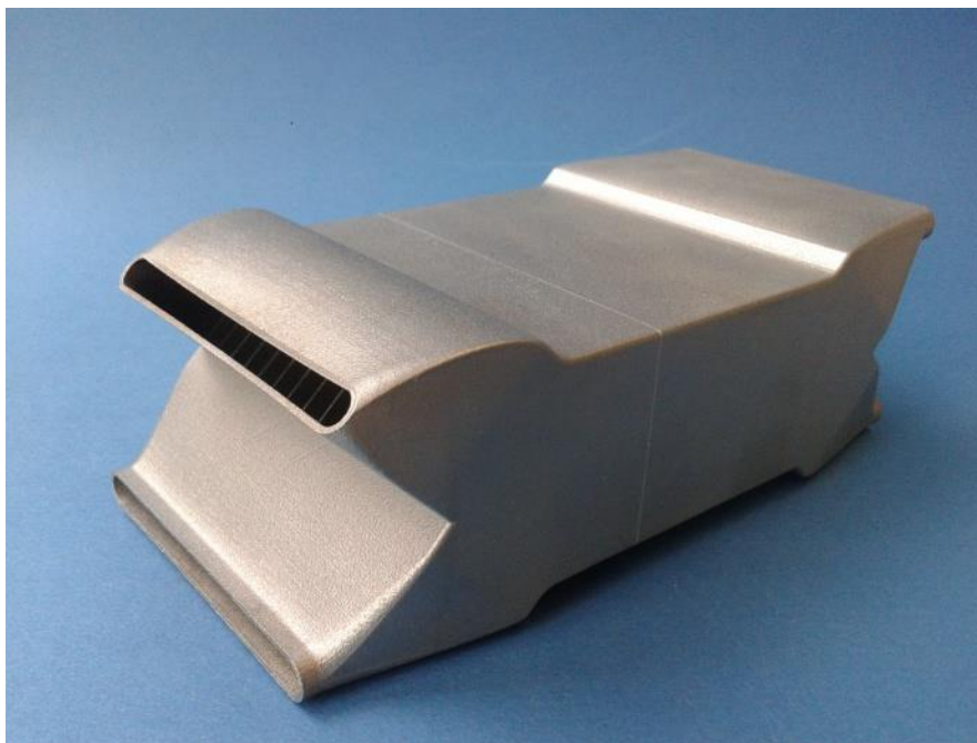
Fig. 6-18: Counterflow heat exchanger manufactured by the use of LBM
