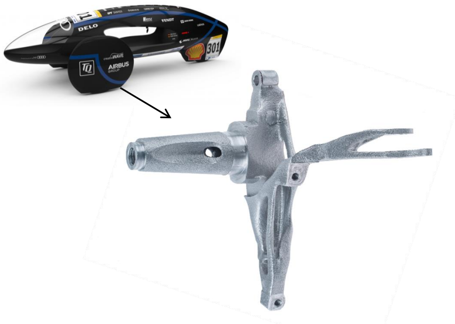
Fig. 6-1: Bionic wheel carrier manufactured by the use of LBM
