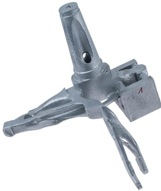
Fig. 6-7: Design 3 prior to mechanical post-treatment (milling) with foreseen design adaptations and clamping region
