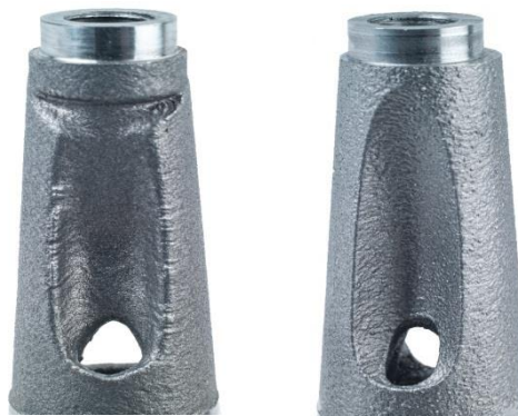
Fig. 6-6: Comparison of transition regions of STL-based Design 2 (left) and NURBS-based Design 3 (right)
