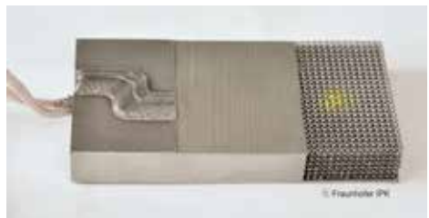
Figure 2: Laser Metal Deposition to encase the integrated electronics (© Fraunhofer IPK)
