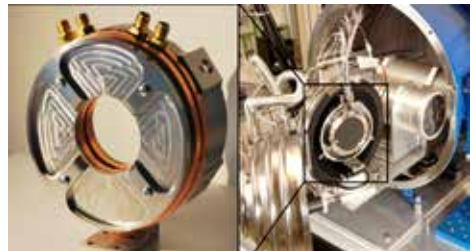
Figure 2: Left: Assembled specimen holder unit with additively manufactured copper alloy parts. Right: Emissivity measurement facility at PTB in Berlin. (© Fraunhofer IPK)
