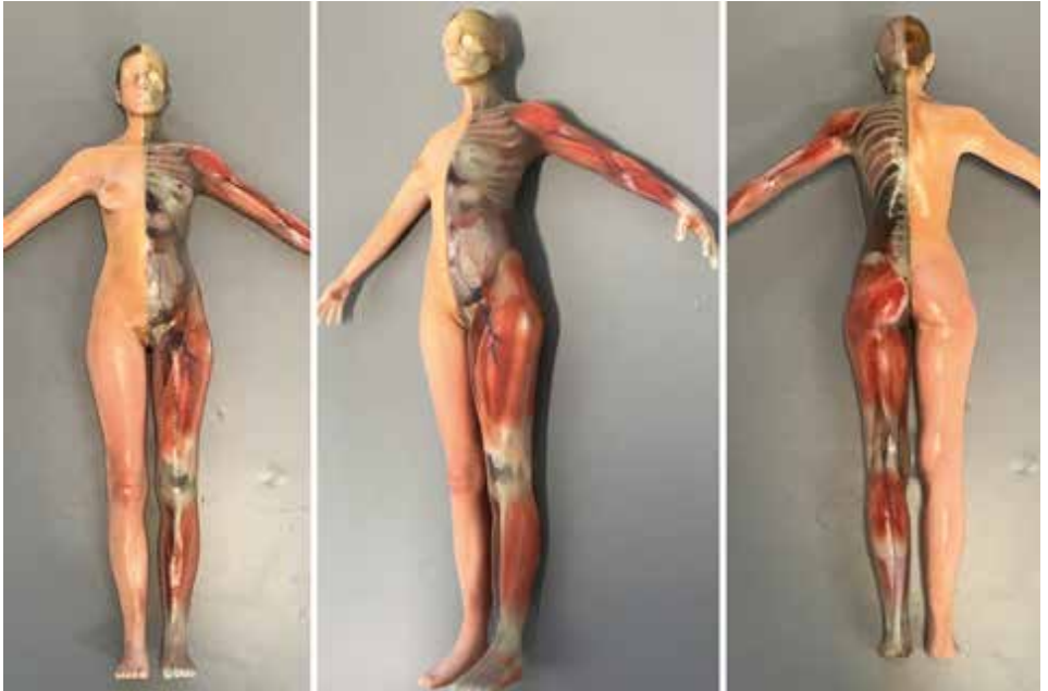
Figure 1: Cuttlefish turns complex models with multiple sub-parts and RGBA textures into 3D prints with highly accurate color and translucency. (© Fraunhofer IGD)
