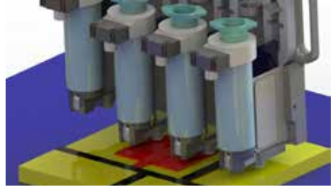
Figure 1: T3DP testing facility with four installed microdispensing systems (© Fraunhofer IKTS)
