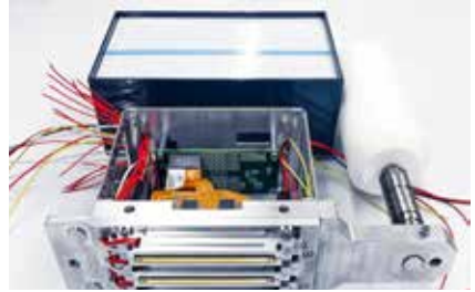
Fig. 2: Printing system containing 3 printing units, 2 UV-led light sources for pinning and a flattening unit (left); detailed bottom-view of printing unit (right) (© Fraunhofer IPA)
