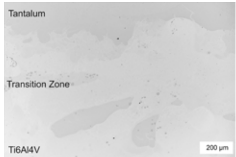
Fig. 3: Sharp material transition Ta/Ti6Al4V (© Fraunhofer IWS)
