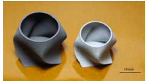
Figure 2: Twisted box (stainless steel 316L, green and sintered) (© Fraunhofer IFAM)
