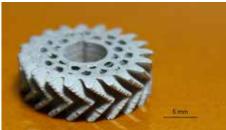
Figure 1: Printed and sintered gear wheel (© Fraunhofer IFAM)
