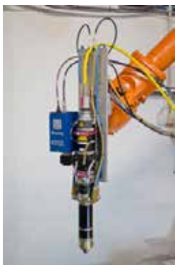
Fig. 1: Powder-based multi-material LMD processing (© Fraunhofer IWS)
