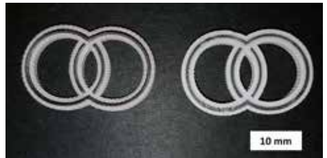
Figure 2: co-sintered zirconia component (black and white ZrO 2 ) (© Fraunhofer IKTS)
