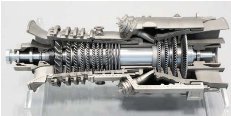
**Technological demonstration model "Siemens SGT6-8000H", scaled model in a gas turbine for power generation. It was produced entirely by additive processes.**
